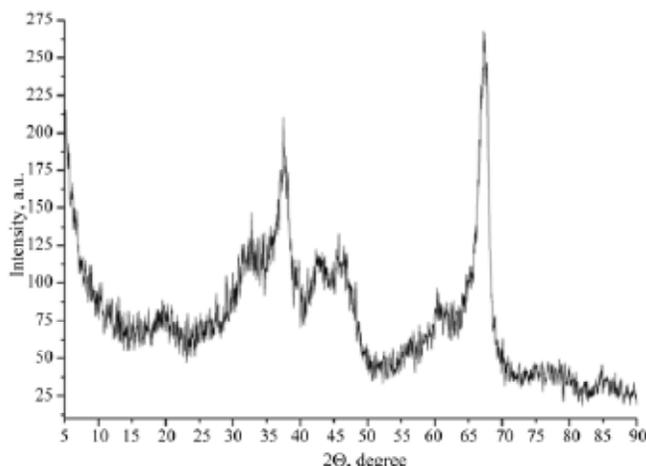
Fig. 2. Diffractogram of alumina micropowder after annealing at 800°C
