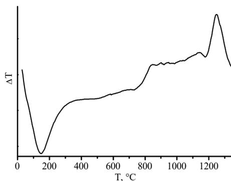
Fig. 1. DTA curve for alumina micropowder
