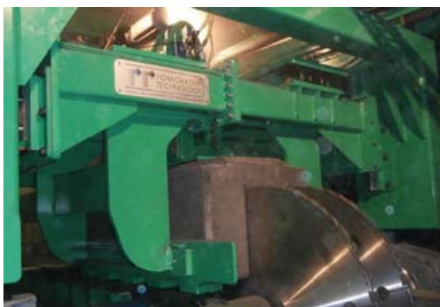
Fig. 4. Last generation of Automatic Anodes Slotting Machine in operation
