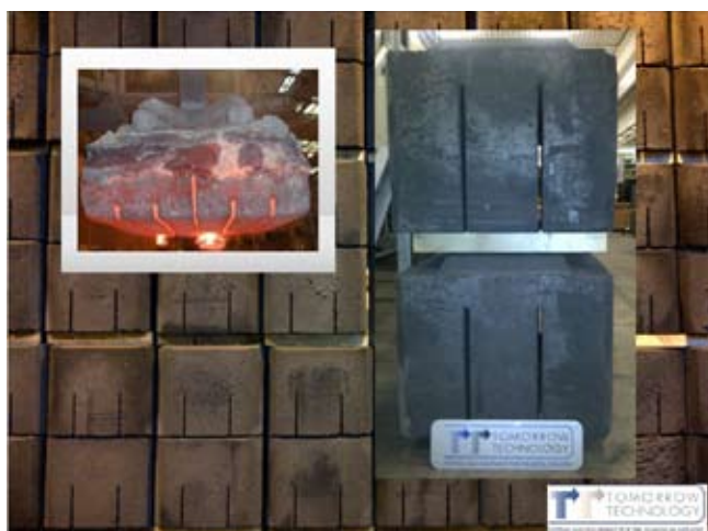
Fig. 5. Slotted anodes at end of life and before being put in operation
