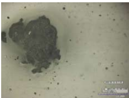
Fig. 10. A carbon-black particle. 1400 \times microscope magnification
