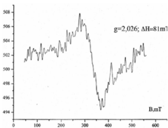
Fig. 20. The EPR spectrum of diamond-bearing carbon-black after cavitation processing
