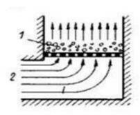
Figure 1 shows a combustor where a fuel dense layer (1) is burned in a layer which lies on a grate and the air is blown (2) upwards. This method is used in boiler units with the capacity up to 40 t/h of steam. Lignite, black coal, semi-anthracite, sod peat, oil shale and wood waste are burned in this way.
