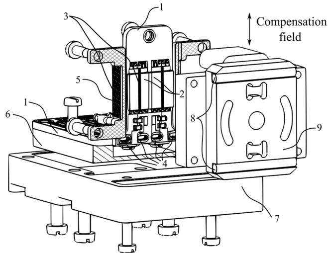
Fig. 3. Weak magnetic field sensor design (1 – PCB; 2 – thin magnetic films; 3 – microstrip transmission line; 4 – via-holes; 5 – compensation coil; 6 – electromagnetic shield; 7 – device enclosure; 8 – magnets; 9 – holder)
