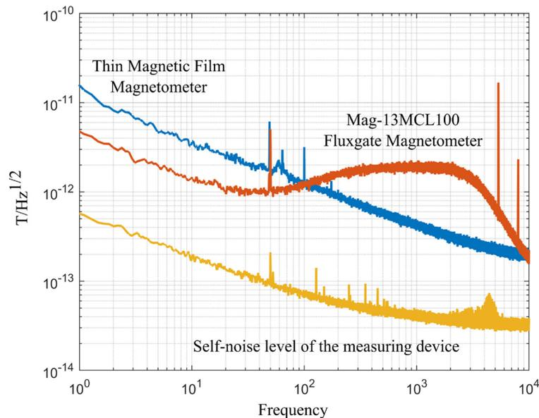
Fig. 4. Self-noise level of the device
