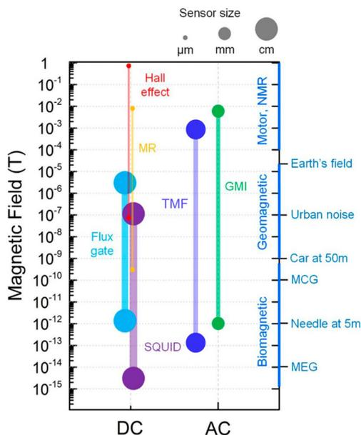
Fig. 1. Comparison of the measurement range of magnetic field sensors [2]
