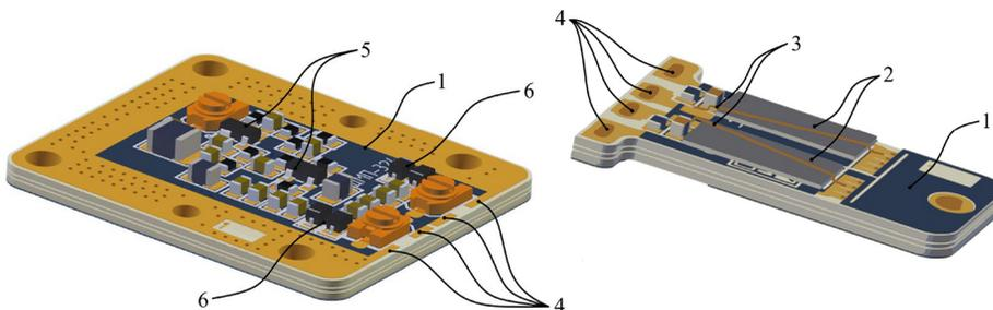
Fig. 2. PCB of microwave oscillator (a) and resonator (b) (1 – PCB; 2 – thin magnetic films; 3 – microstrip transmission line; 4 – via-holes; 5 – microwave oscillator; 6 – amplitude detector)
