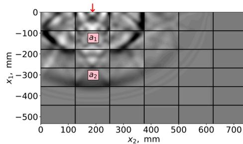
Fig. 5. The numerical experiment diagram. Accelerometers  $a_1$  and  $a_2$  are placed in the central points of the corresponding blocks
