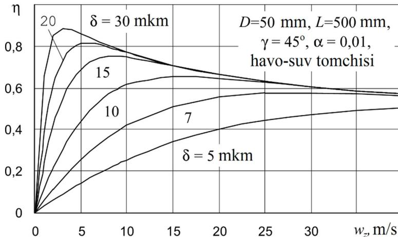
Fig. 2. A graph of the calculated dependence of the separation efficiency on the flow rate when taking into account the secondary removal
