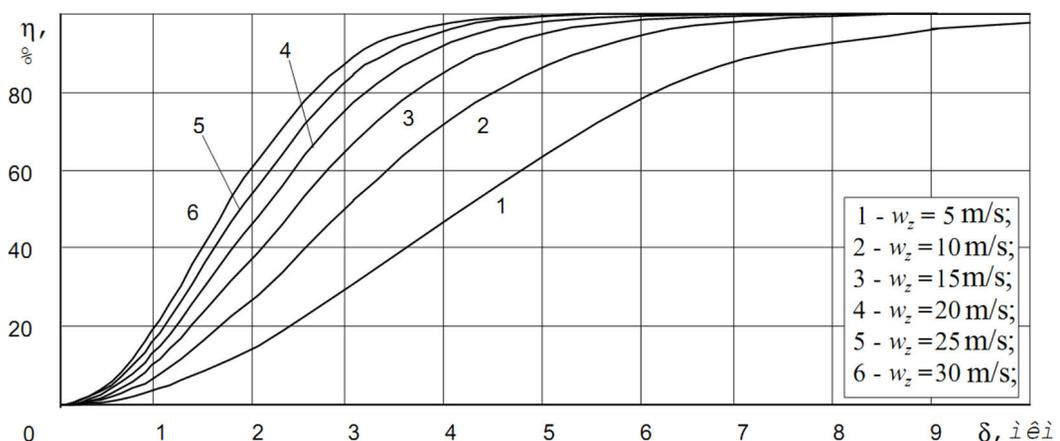
Fig. 1. Calculated fractional efficiency of centrifugal separation without secondary extraction: air-water 20 °C,  $D = 30$  mm,  $L = 300$  mm,  $g = 45^\circ$  system when
