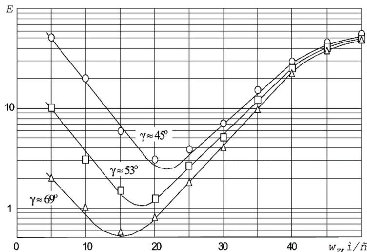
Fig. 3. Dependence of the displacement of the dispersed phase on the axial velocity and the angle of the twisting current: M-1 quartz powder at an ambient temperature of 80 °C; the concentration of the particle is  $10^{10} \text{ m}^{-3}$ ; particle diameter  $0.1 \div 5.0 \mu\text{m}$ ; the temperature of the cooling agent is 10 °C; specific consumption of steam is 0.1 kg/kg
