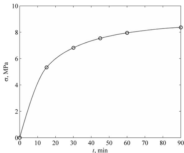
Fig. 4. Dependence of the maximum normal temperature stresses in the anode block on time
