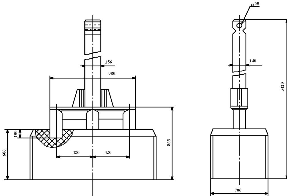
Fig. 1. The anode block of the industrial electrolytic cell
