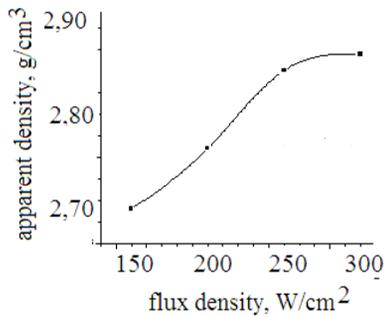
Fig. 1. Dependence of apparent density of pyroxene material samples on flux density
