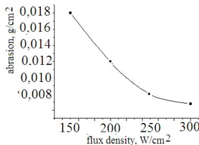
Fig. 3. Dependence of the abrasion of the pyroxene material on the flux density
