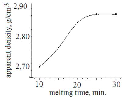
Fig. 2. Dependence of the apparent density of pyroxene material samples on the melt holding time at 300 W/cm<sup>2</sup>
