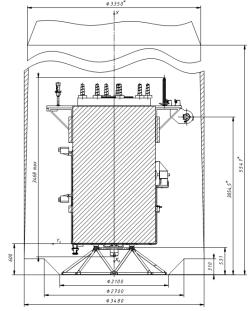
Figure 2 - Placing the SC-FD into the booster
