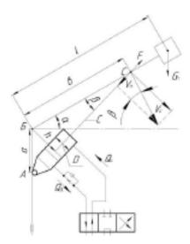
Figure 1. The design scheme of lowering the boom lifting mechanism.
