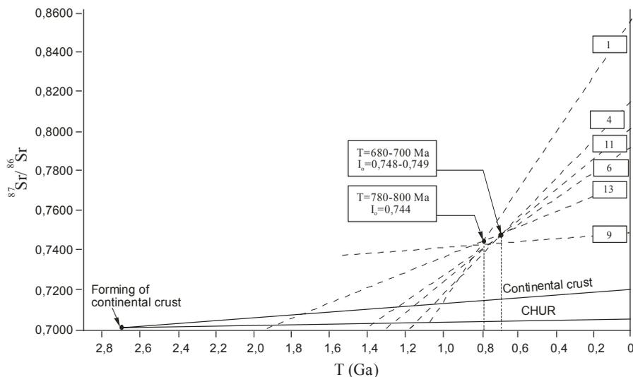
Fig. 7. Evolution of  $^{87}\text{Sr}/^{86}\text{Sr}$  ratio in whole rock samples from the Blagodat deposit (numbers of samples from 1 to 18 corresponded to the table 3) demonstrated Sr model ages of rocks relative to the average composition of upper crust. Numbers of samples from 1 to 18 corresponded to the table 3
