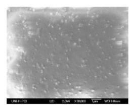
Fig. 2. A sample of water-soluble paint with immobilized silver nanoparticles
